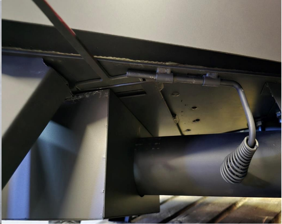
Pellet Breach Tool Damper Lock / Stop Position @ lowest setting. Move to slide closed.
